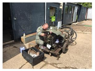
Our hydraulic rig, which is used for testing aircraft hydraulic systems, is powered by a Coventry Victor engine which has become increasingly difficult to start in recent years. This is now the subject of an ongoing overhaul, probably the first real attention it has had since it arrived in Wellesbourne many years ago. Once this has been completed, we will be able to continue our investigations into the nose wheel steering deficiencies mentioned by Mike in his introduction.
