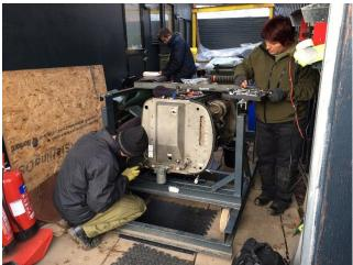
The alternator was removed and examined, and the only fault found was that the field brushes were rather tight in their housings due to an accumulation of carbon dust. They were cleaned up and the spring tensions were measured and found to be ok. We then re-assembled the AAPP and refitted it to the aircraft.
