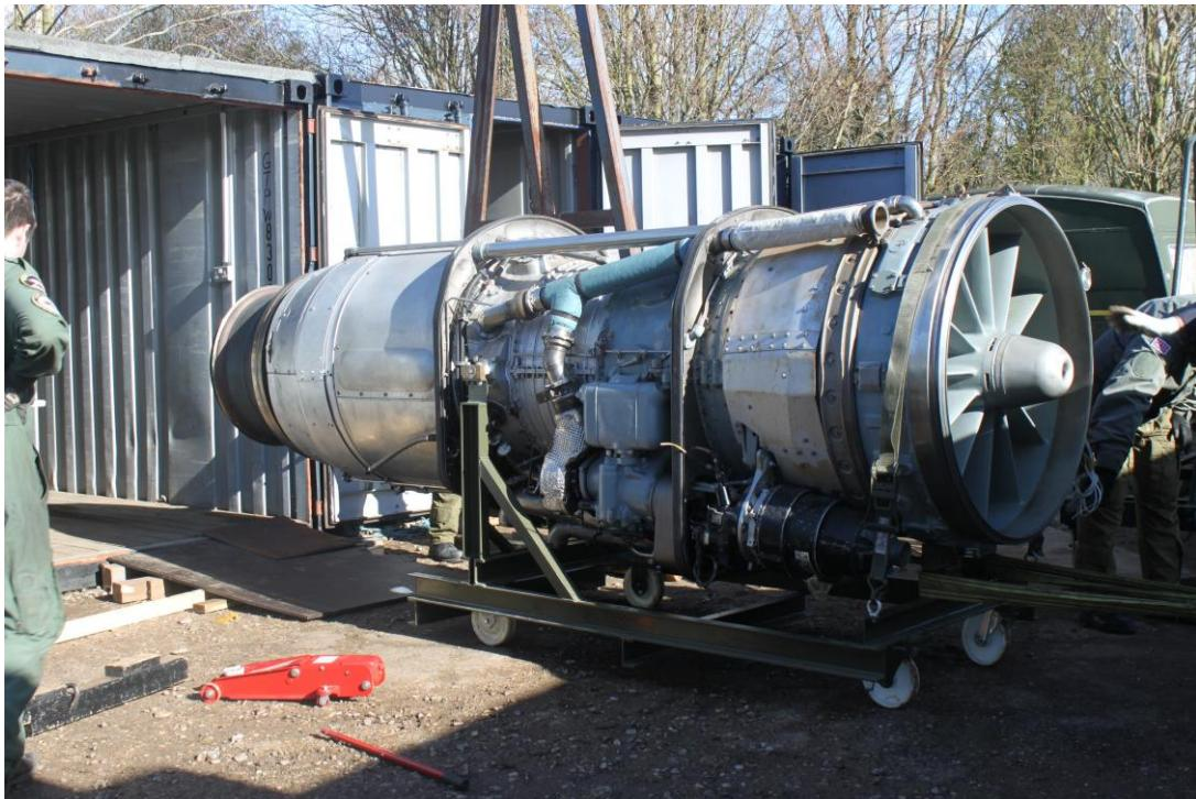
This has now been completed and an EGR carried out, and we are pleased to report that the “new” engine, which hadn’t run for probably thirty years, performed faultlessly. We will dismantle and inspect the turbine end of the removed engine, and also address the fuel system problem, after the busy summer period is over.
