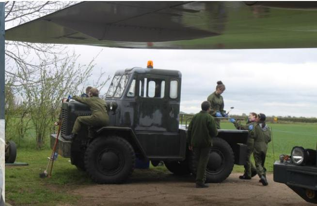
The Coleman was also the cause of much head-scratching when the engine started to misbehave. As the picture shows, it drew a lot of attention, and a lot of different proposed solutions, but the problem was eventually located in the carburettor. A good clean and rebuild and all is now serviceable again.
