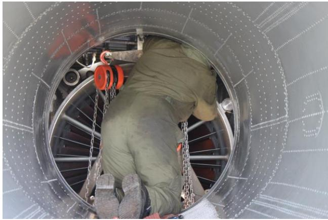
Here Roger is preparing the mounting and access is already very restricted, and at this point the engine still has to be hoisted a further 10 inches or more.
