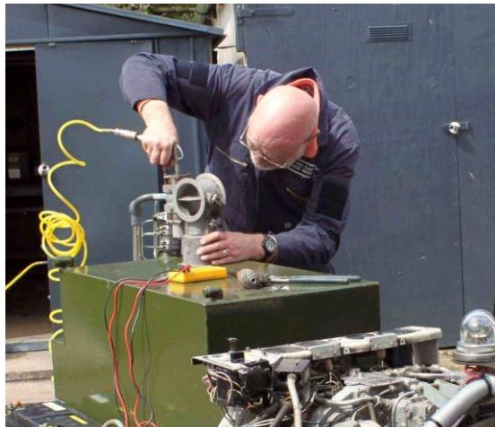
Another item of ground equipment which has given a couple of problems of late has been the Palouste air starter. Initially, we thought the fault was in the cable connection from the aircraft, but diagnosis showed it was actually an air delivery valve defect. Strip and rebuild of the valve proved ineffective, and the problem was resolved by fitting a spare unit.
