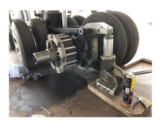
Also on the aircraft, all of the main landing gear wheels have been removed for inspection of the brake packs. One pack was removed to the workshop to have its hydraulic seals renewed, and then refitted. We also had to renew the seals in several of the walking joints which allow the brake pipes to accommodate the movement of the undercarriage, and all the brakes are now in satisfactory condition.
